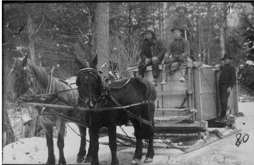
Image 1. “The sprinkler or watering box.” (Source: Image published with permission from the Patten Lumbermen’s Museum.)
