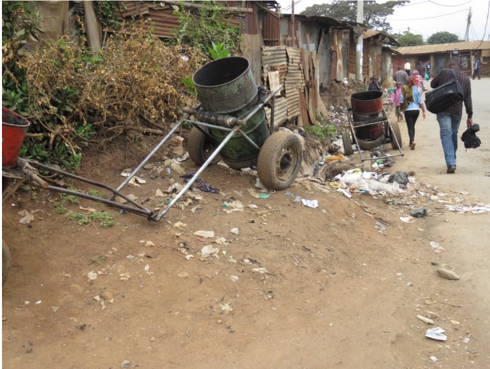
Figure 2. Localized push/pull cart pit-latrine hand-emptors in Kibera Informal Settlement, Nairobi, Kenya. (Photo by author, 2016.)
